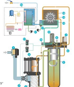
Intake air Air/oil mixture Oil Inlet filter Sentinel valve Interior permanent magnet motor (iPM) Air/oil vessel Thermostatic bypass valve Oil filter Safety valve Oil separator Solenoid valve After-cooler Oil-cooler
