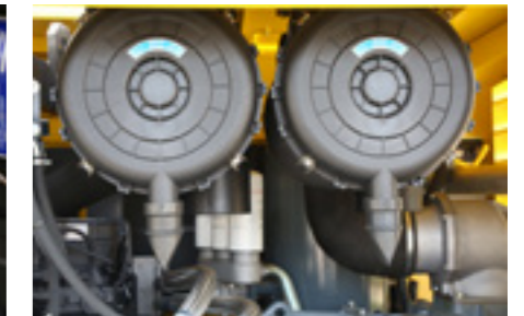
Heavy duty air filter with safety cartridge as standard.
