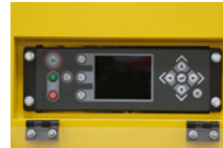
XC2003 controller with IP65 protection and easy operation*.
