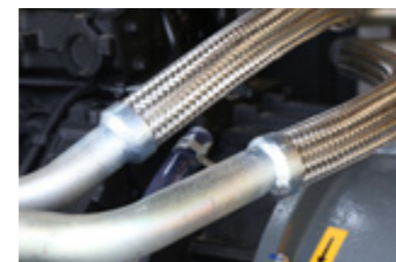
Metal braided hose to improved safety and longevity.
